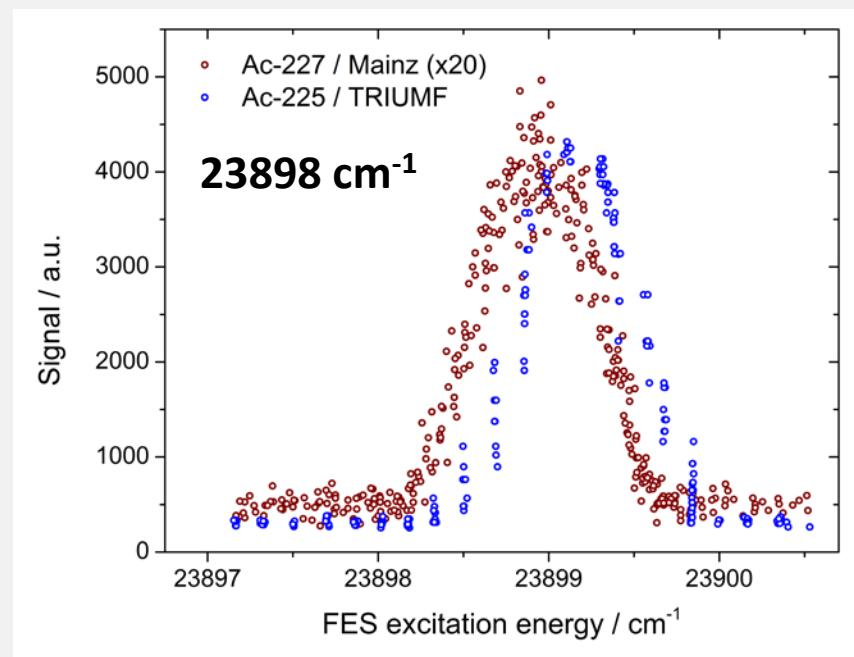
About 0.2 cm<sup>-1</sup> (6 GHz) isotope shift  $^{227}\text{Ac}$ - $^{225}\text{Ac}$  measured
