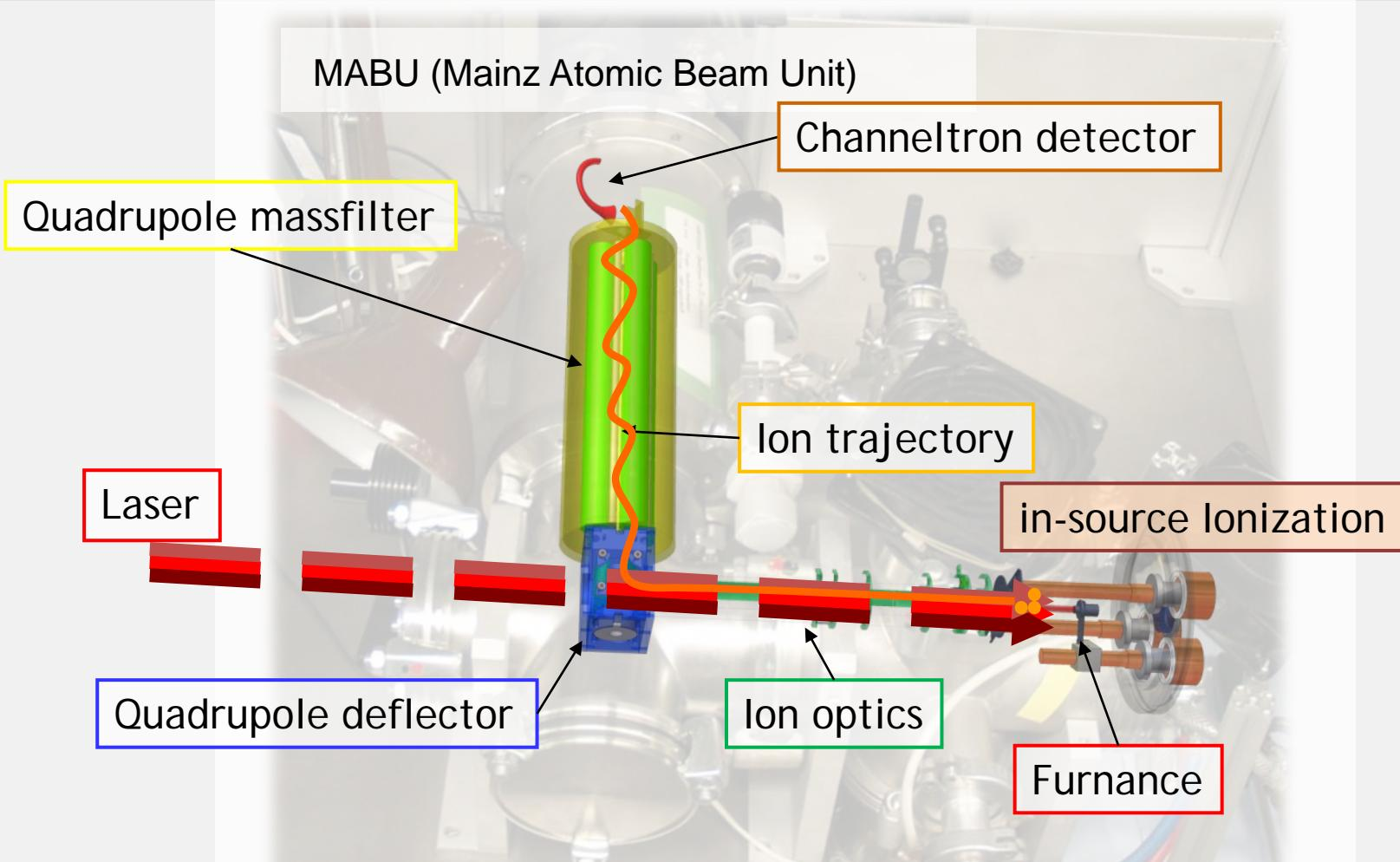
Laser ion source & laser in-source spectroscopy
